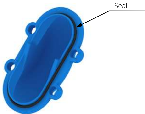
Fig. 5. Placing of the o-ring type seal on the circumference of the valve cover
