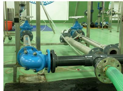
*Tested valve on a testing system, in a recumbent position*
